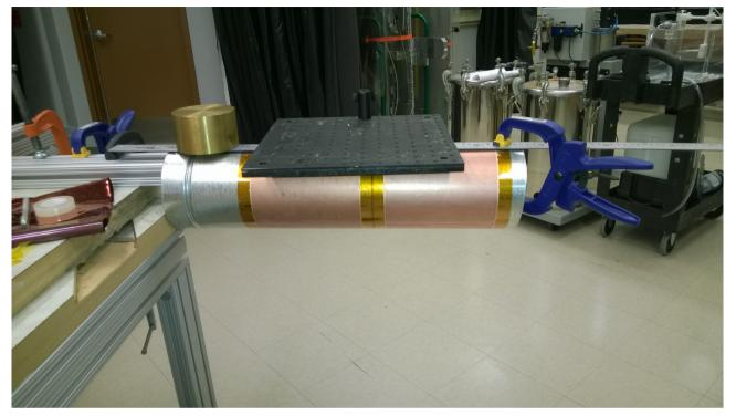
GEM foil Wrapped on the cylindrical structure
